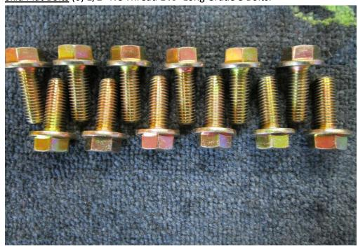
• Steering Box Bolts (3) 7/16" NC Thread 3" Long Grade 8 Bolts. (3) 7/16" Flat Washers
