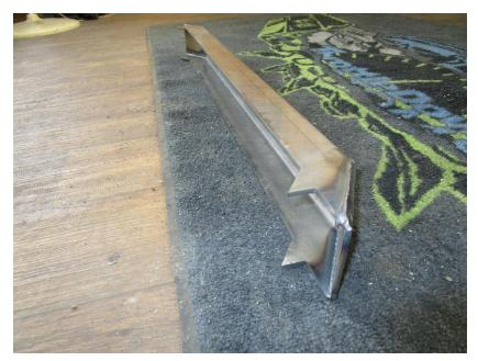
We also supply a new Rear Tank Strip that may or may not need to welded into your Factory Frame.
